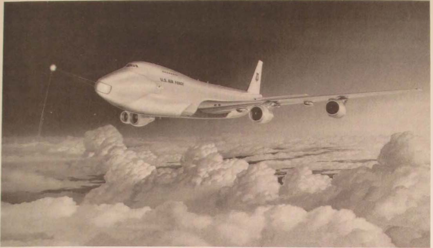
In the airborne laser, the Air Force stands to gain a silent, very long range, speed-of-light weapon. These contractor versions of ABL weapon system platforms are part of an Air Force Advanced Technology Transition Demonstrator program to develop and demonstrate technologies for tracking and killing theater ballistic missiles during boost phase.
